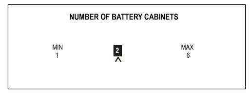
Set the number of battery cabinets by changing the number in the highlighted box. Pressing SELECT will save this information and return Operator to the System Settings Screen.
